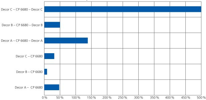
Resistance values of the 1 mm lines compared to Brecton<sup>®</sup> CP 6680 an PC film [ $\Delta R$  %]
